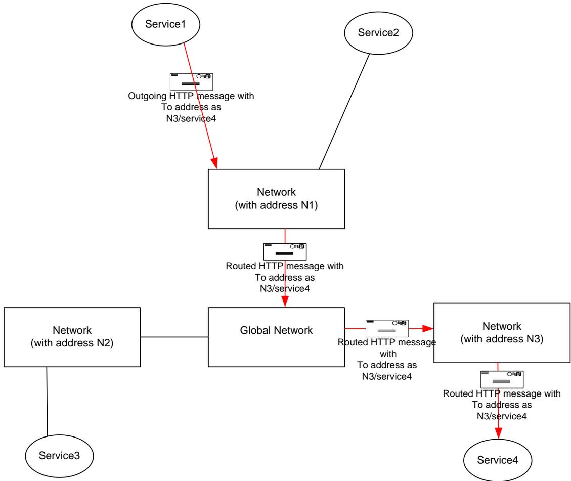
**Figure 3.3 Inter-network type service communications**
