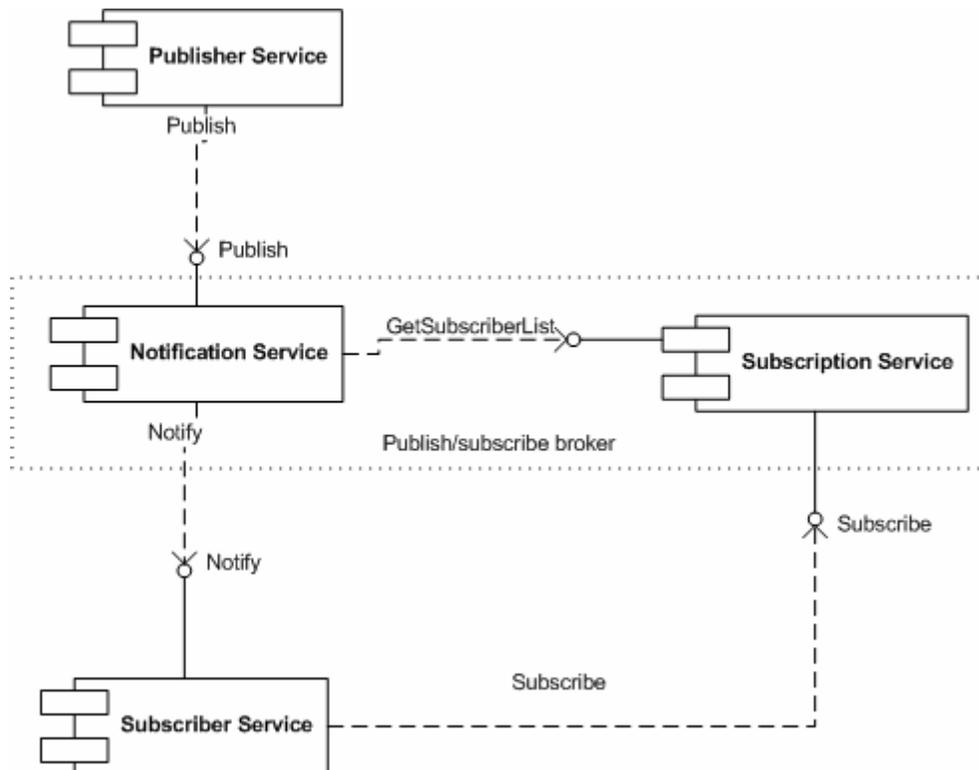
**Figure 3.4 UML Component model of a publish/subscribe broker service and its relationship with publisher and subscriber services.**
