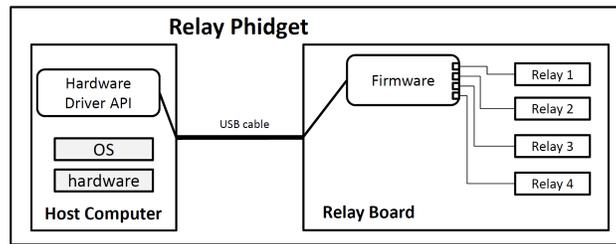
Figure 1: Relay Phidget as a computational-physical system
