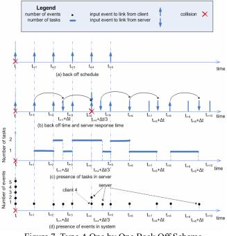
Figure 7. Type A One by One Back Off Scheme
