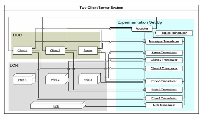
Figure 5. System Decomposition of a Two-Client/Server Network
