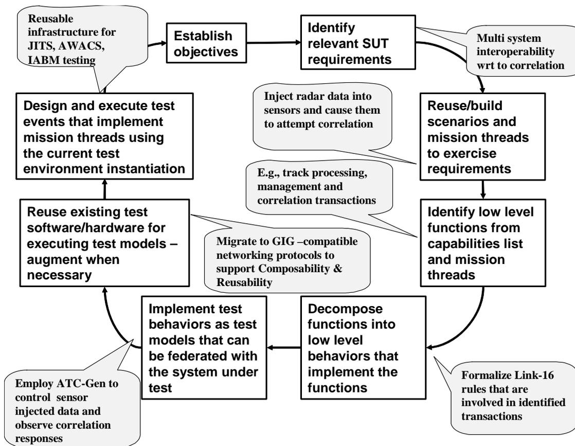
Figure 6. Illustrating Event Planning Cycle for Sensor Simulation Acquisition
