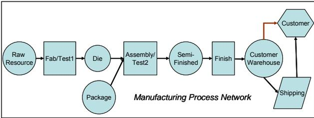
Figure 1: Semiconductor Manufacturing Process Network
