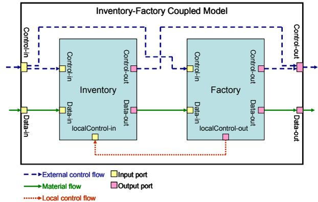
Figure 3: Structural Composition of Inventory and Factory Models
