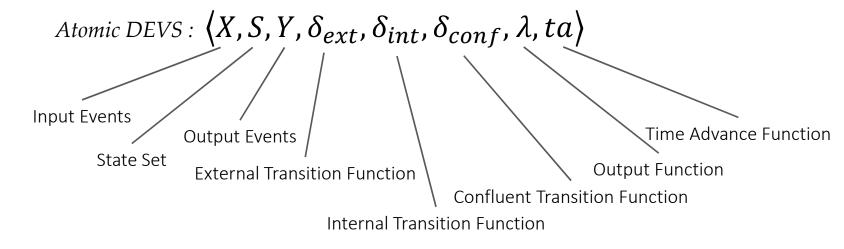
$ta: S \to R_{0,\infty}^+$  $\delta_{ext}: Q \times X \to S \text{ where } Q = \{(s, e) \mid s \in S, 0 \le e \le ta(s)\}$
